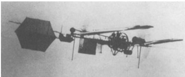
Before attempting a full-scale version, Langley built a quarter-size model that flew successfully in 1901. It was the first time a gasoline engine had driven an airplane.
