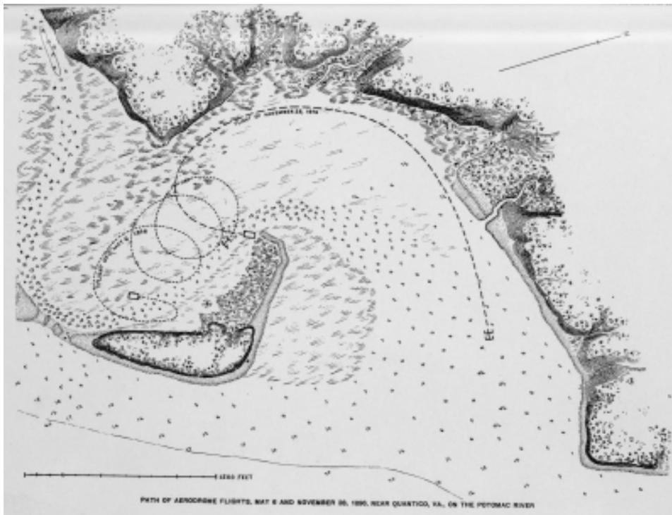
Path of Langley's experimental aerodrome flights on May 6 and November 28, 1896, near Quantico, Virginia, on the Potomac River. From Langley's memoir on mechanical flight. Part I: 1887-1896.
